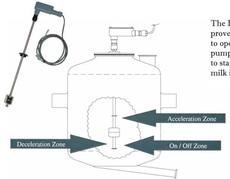
The ImPulse III uses proven float technology to operate the milk pump at variable speeds to stay just ahead of the milk inflow rate.
